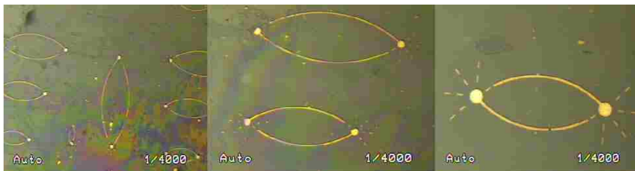
Figure 5-2: Metallized image of the two-neuron circuit design with different dimensions
