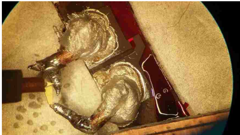
Figure 6-1. Device showing the electrical connection to the bond pads using conductive epoxy to copper wire leads.
