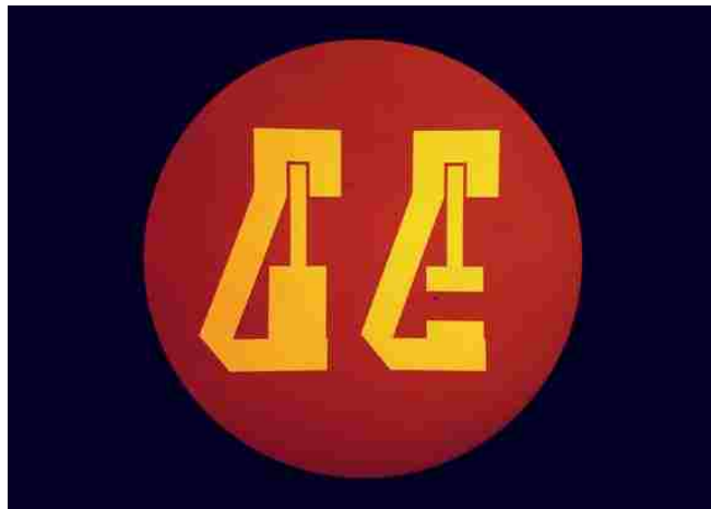
Figure 4-3. Open (right) and approximately shorted (left) probe pad structures used for parasitic extraction.
