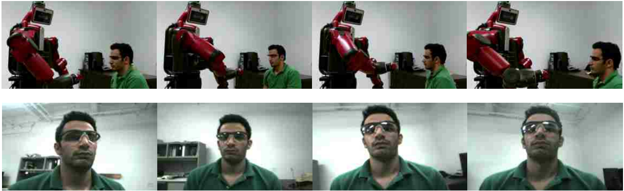
Figure 3.6: Sequence of images demonstrating the execution of the tasks of recording a video of subject's face for facilitating a video chat. The top row shows the relative position of the user and the Baxter robot, while the bottom row shows the video captured. Notice that although the user had moved around significantly, his face remains centered in the video stream.
