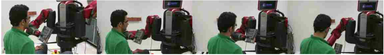
Figure 3.5: Sequence of images demonstrating the task of holding a book for the user to read. Notice that as the the user turns his head, the robot positions the book for a comfortable reading position at an appropriate reading distance.
