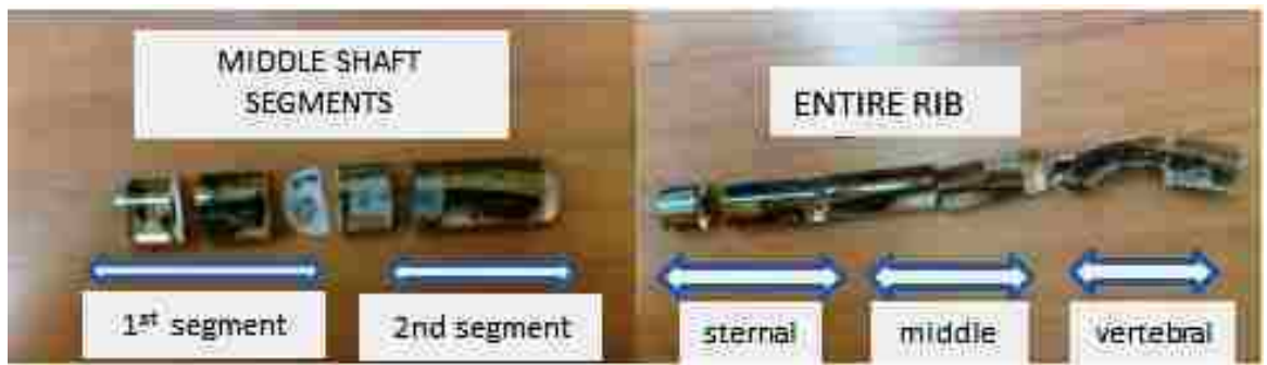
Figure 4.7 Preparation process for the pilot study sample: segment cutting for the extraction of six sections per rib (study sample).
