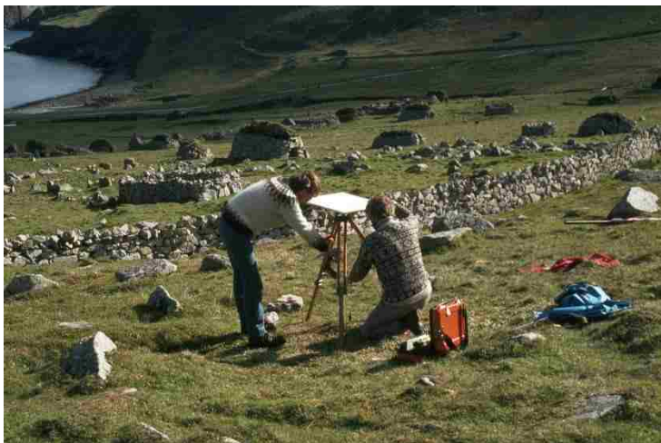
Figure 11 RCAHMS staff setting up a plane-table in 1983. DP220795
