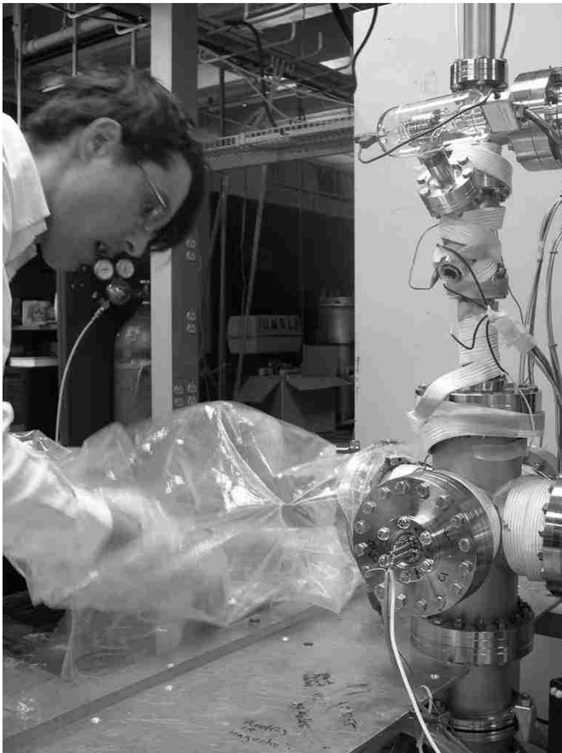
Figure 2.5. Use of the glove bag. Electrical feedthroughs for thermocouples and high temperature stage heater, heat tape for top and bottom chambers, and aluminum frame for supporting the system and glove bag are shown.
