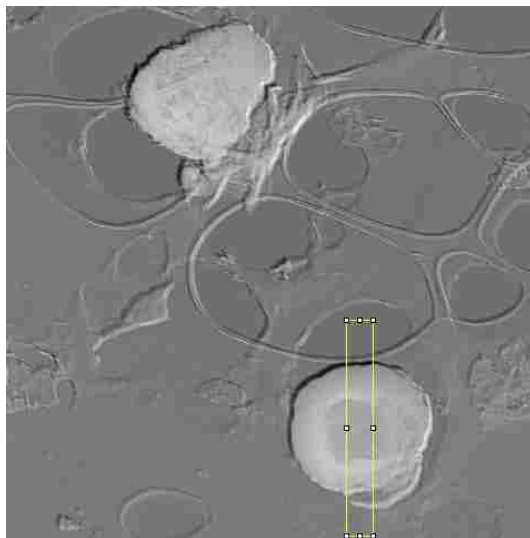
Figure 5.4: A calculated mean-free-path thickness image of a graphite spherule with a nanocrystalline core (field of view \sim 4 [microns]). Variations in intensity are indicative of mean-free-path differences. The windowed region corresponds to the profile shown in Figure 5.5.
