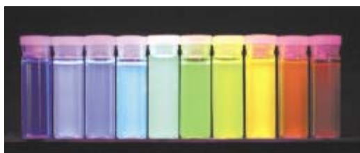
Figure 1.1. Ten different emission colors of different size ZnS-coated CdSe nanoparticles excited with a near-UV lamp. From left to right (blue to red), the emission maxima are 443, 473, 481, 500, 518, 543, 565, 587, 610, and 655 nm, respectively. Reprinted with permission from [15], M. Y. Han et al., Nature Biotechnol. 19 , 631 (2001).
