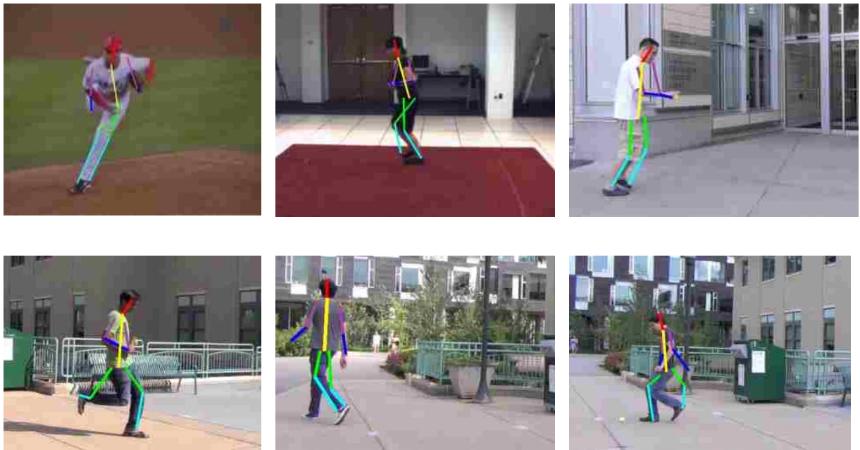
Figure 5.19: Failure Cases. Some of the failure cases are caused by occlusion (1-3), and some are caused by failed detection of joints (4-6).
