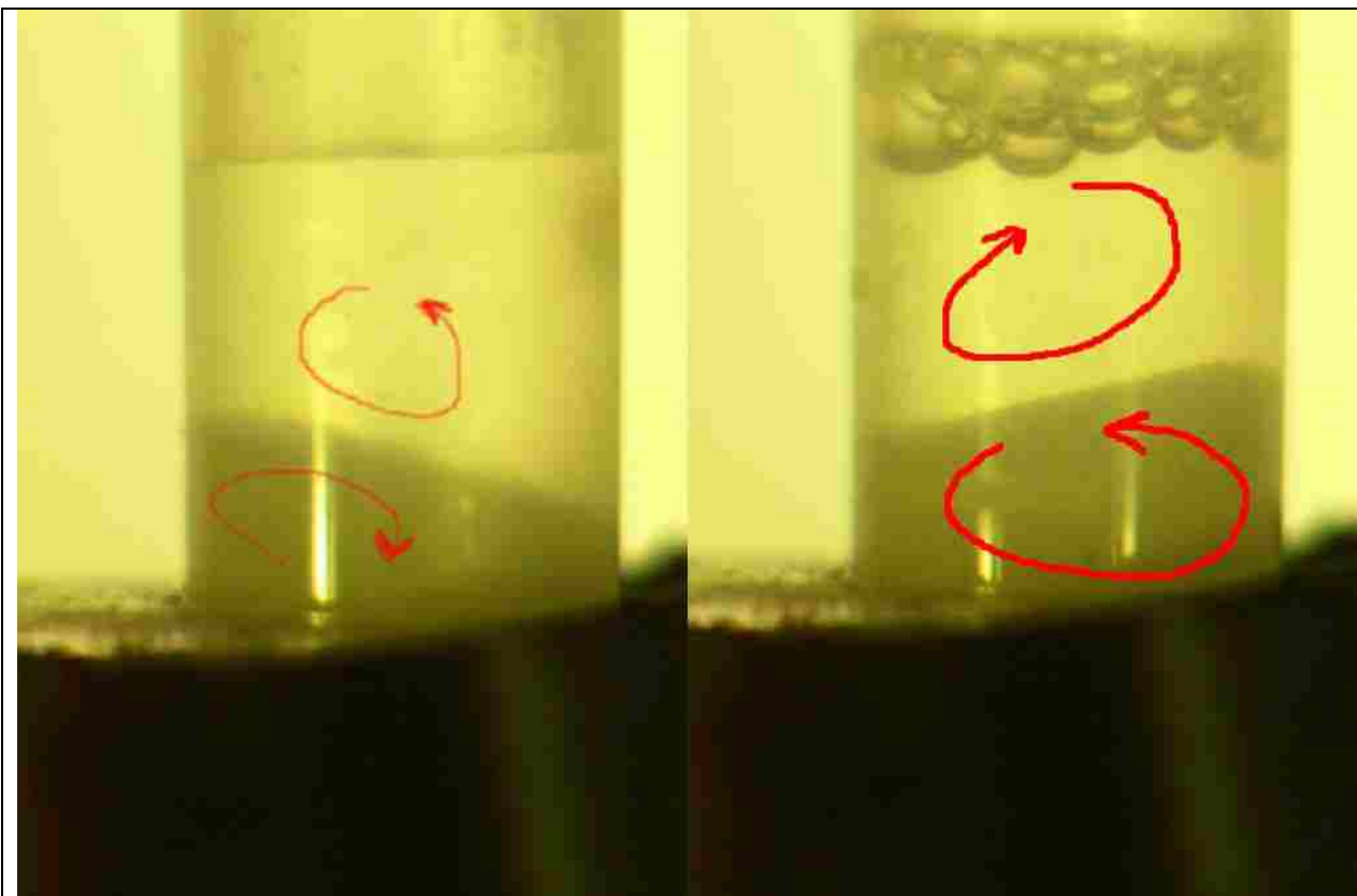
Figure 131: Comparing AudioLyse bead slurry movement with (right) and without (left) micro90 surfactant. The only superficial difference apparent in the videos was the presence of the bubbles at the top of the tube with the micro90, present due to vibration while the magnet, beads, micro90 and water were added.
