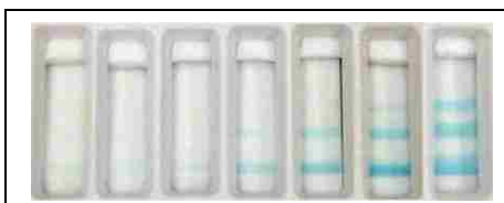
Figure 8. Ladder-bar readout for a glucose assay demonstrated by Fung et al. [43]. A sample consisting of 0, 1, 5, 25, 50, 100, and 200 \mu\text{m} glucose was added to the strip, from left to right, respectively.
