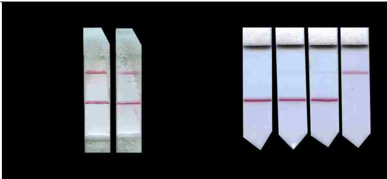
Figure 101: Detection results excerpted from dry storage study. (a) Prototype iSDA and LF detection on MRSA genomic DNA input using pads stored for six weeks at laboratory ambient temperature in desiccated conditions. Duplicate tests confirm dry reagent viability in these conditions through Idh1 amplification and detection functionality. (b) Manual assay tests on low input copy number MRSA genomic DNA using pads stored for 15 days at 40^{\circ}\text{C} in desiccated conditions. Triplicate tests confirm dry reagent viability in these conditions through Idh1 amplification and detection functionality. Associated negative control indicates no contamination.
