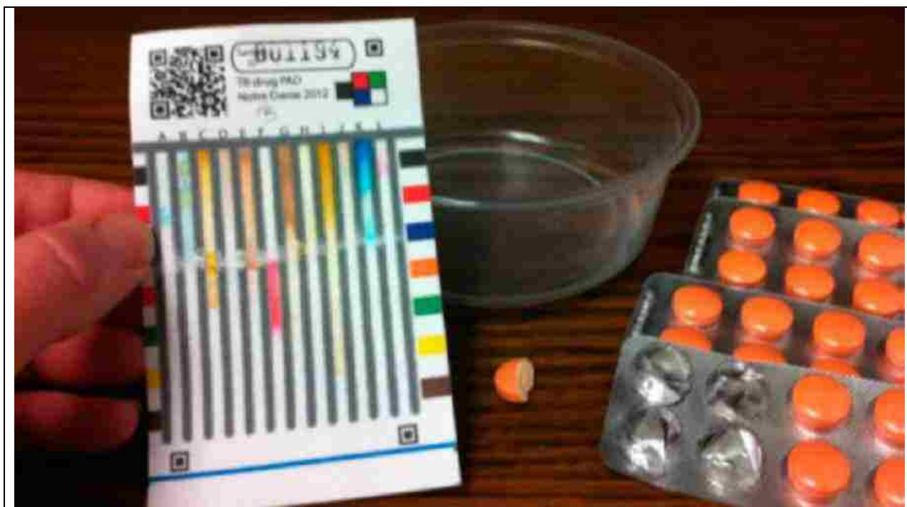
Figure 6: Example of a paper analytical device (PAD) developed by the Lieberman group for counterfeit pharmaceutical testing, in this case for TB drugs[40]. Reprinted from Anal. Chem. , 85(13), 6453–6460. Copyright 2013, American Chemical Society.
