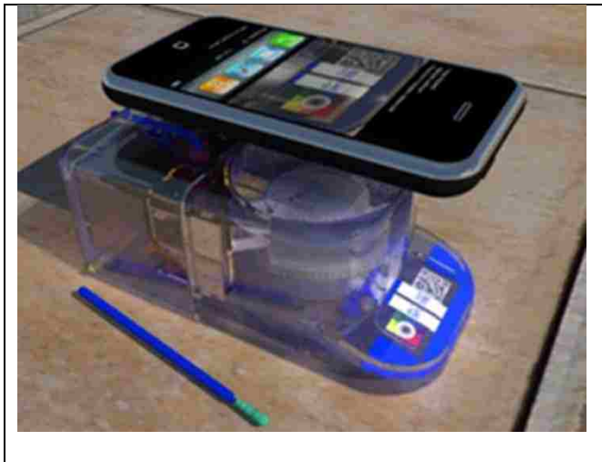
Figure 1: MAD NAAT device. Swab sample obtained from the patient is inserted in the device. The automated assay quantifies nucleic acid sequence of interest. After some time, the cell phone quantifies assay signal. Graphic by Paul Yager.
