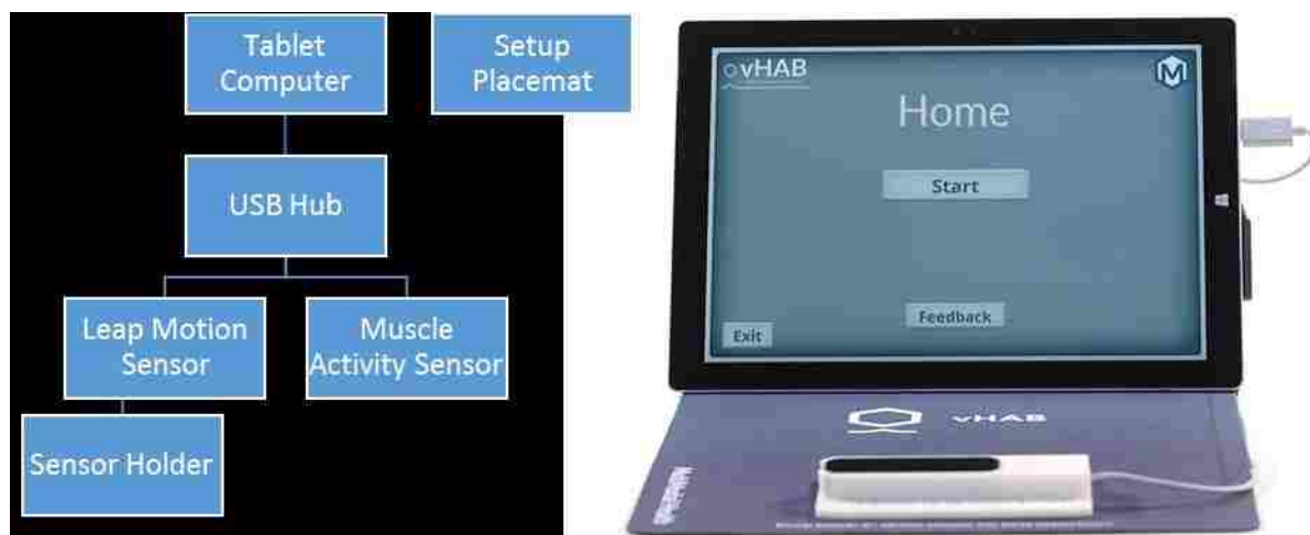
Figure 4.3.1. Block diagram of vHAB hardware components and image of assembled Home system.
