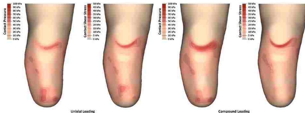
Figure 3.16: Participant three – anterior stresses. Stresses for the compound load profile showed a general increase in contact pressures and resultant shear stresses over the anterior-proximal region. The size of stress distributions over the anterior-distal region were decreased, but only the magnitude of the resultant shear stress decreased while peak pressure over the distal tibia was consistent.
