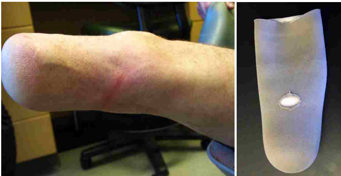
Figure 3.19: Participant three – second skin issue. Participant three also experienced edge loading issues from the posterior brim (a) that were significant enough to tear the fabric backing of his prosthetic liner (b).
