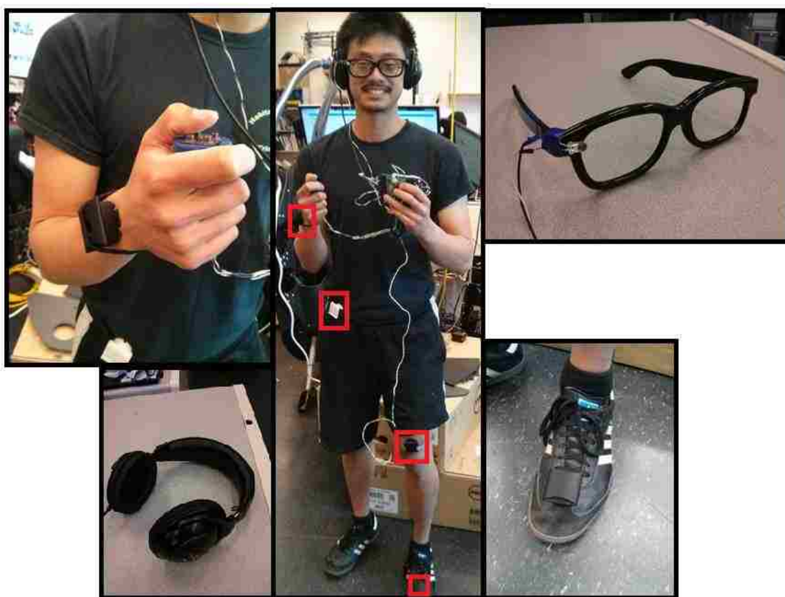
Figure 3.3 – Testing device and placement: Glasses frames with LED and headphones on the head, vibrotactile motors (located at the 4 red boxes), electronics pack held in the non-dominant hand, and response buttons held in the dominant hand.
