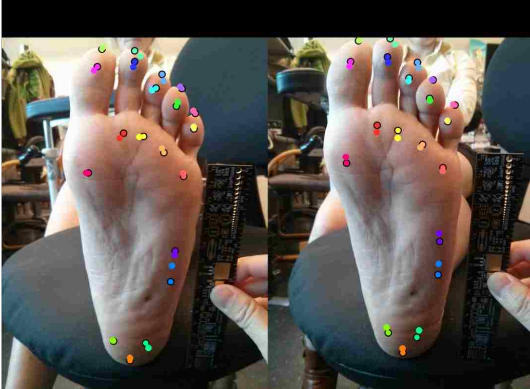
Figure 4.12 – Centroid of ellipses on foot (corresponding color) in relation to actual touched points (black outline).
