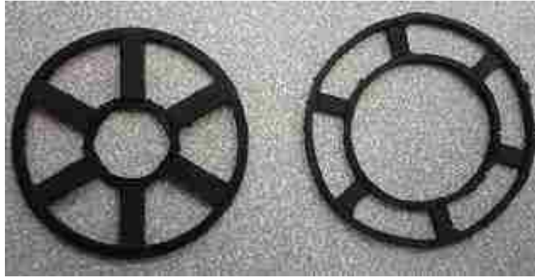
Figure 2.8 – Optimized silicone suspension systems for new LRA (left) and ERM (right) design.
