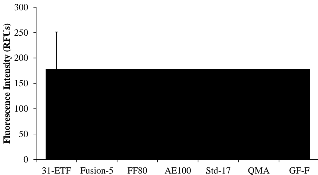
Figure 12. Background fluorescence of selected porous substrates. Intensity values acquired using the Axiovert25 fluorescence microscope with Zeiss 61 HE rhodamine filter set with a 2.5x object at 200 ms exposure.
