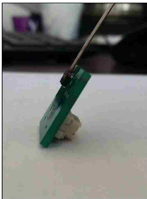
Figure 3.4: Kapton tape applied to the back of the polyimide array makes the device thickness within the recommended upper limit of the ZIF connector without causing device deflection or opening of the ZIF connector.
