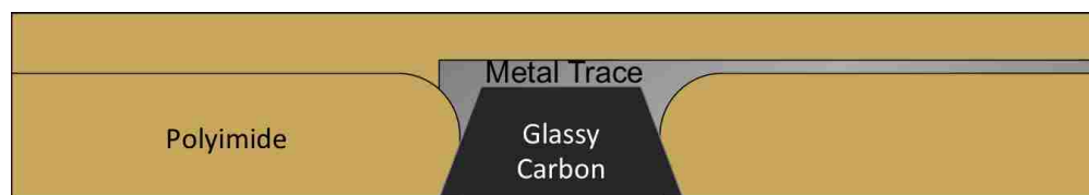
Figure 3.6: Model cross section of a glassy carbon \mu ECoG array depicting what we initially thought the interface between the GC and the metal trace would look like.
