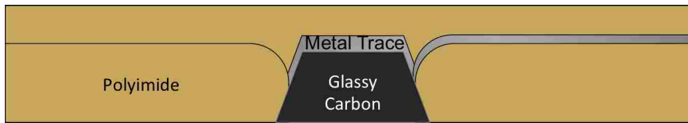
Figure 3.7: Updated model cross section of a glassy carbon \mu ECoG array depicting what the actual interface between the GC and the metal trace would look like.
