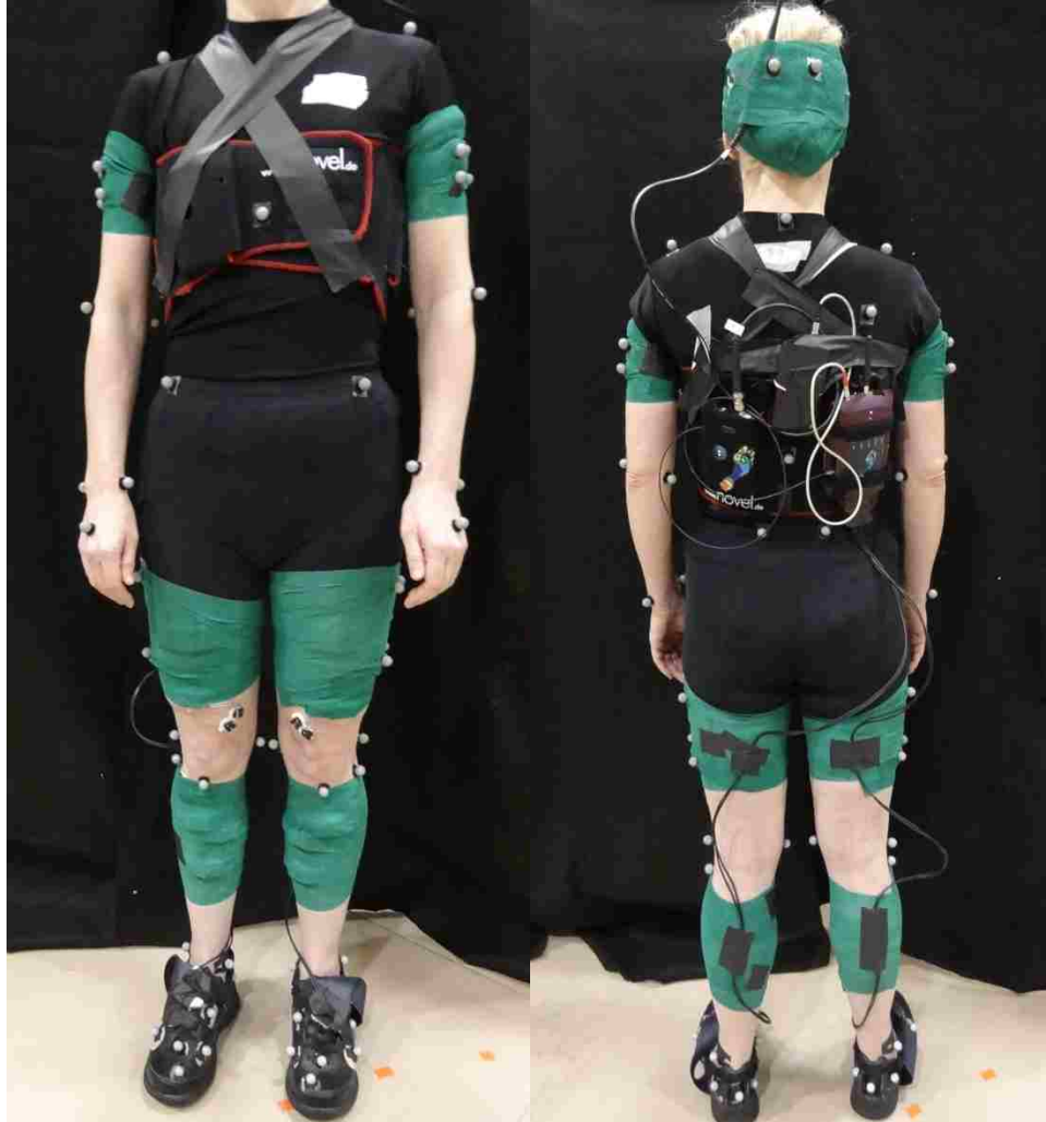
Figure 4 – Fully instrumented participant, equipped with motion tracking and pressure sensing hardware.
