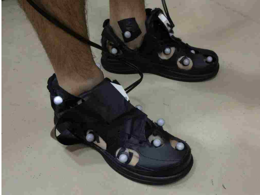
Figure 9 – Instrumented walking shoes with pressure sensing insoles installed.
