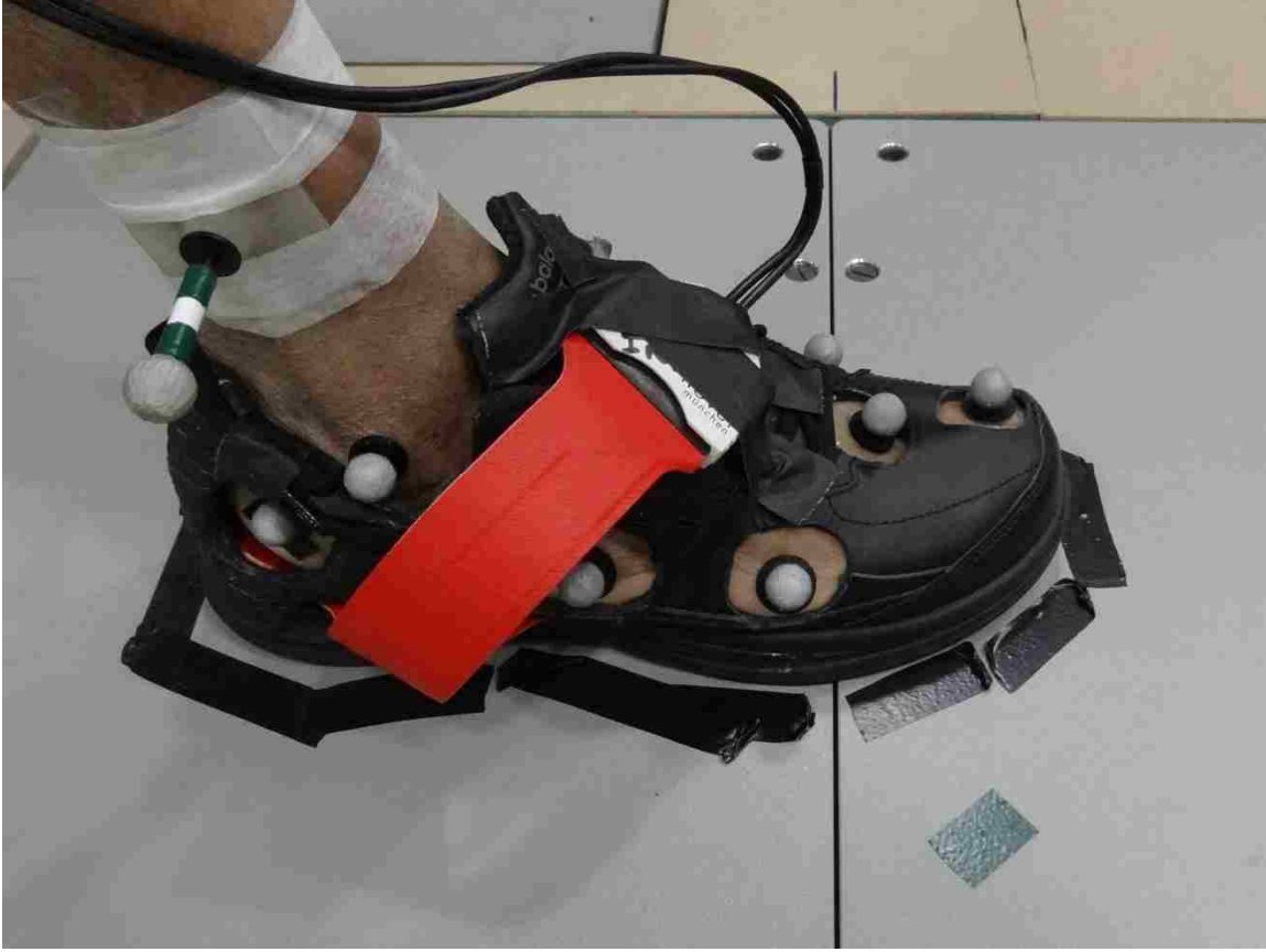
Figure 18 – Shod split plate validation technique. Participant in fully instrumented shoe is shown striking the split plates to validate the MPJ.
