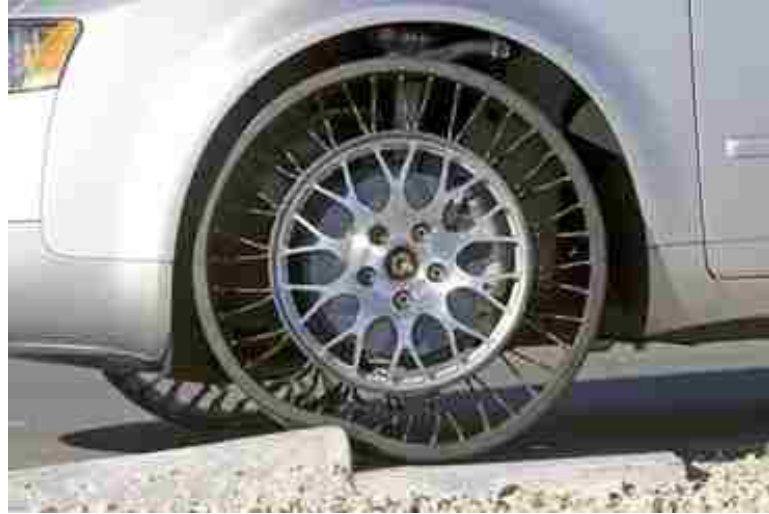
Figure 1.11. Michelin Tweel™ Airless Tire [5]
