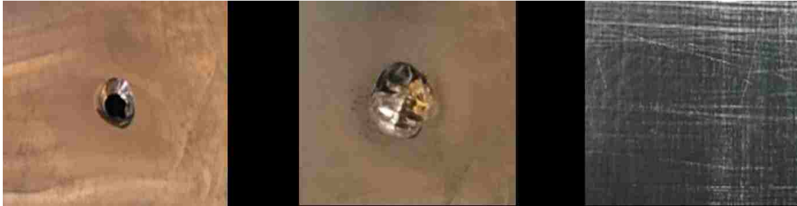
(a) A hole defect on component (b) After deposition (c) After machining and polishing
