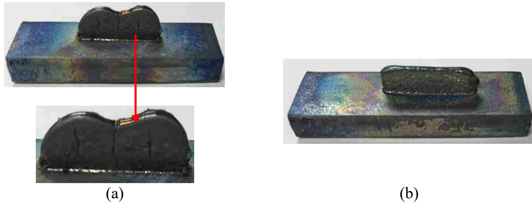
Figure 3.1. Deposited samples in the first experimental design. (a) \gamma -TiAl sample without insulating bricks; (b) 80 wt.% \gamma -TiAl +20 wt.% Ti sample without insulating bricks
