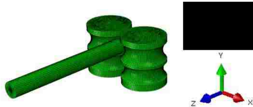
Fig. 10. Modeling of steel bar hot rolling process
