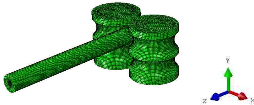
Fig. 8. Modeling of steel bar hot rolling process
