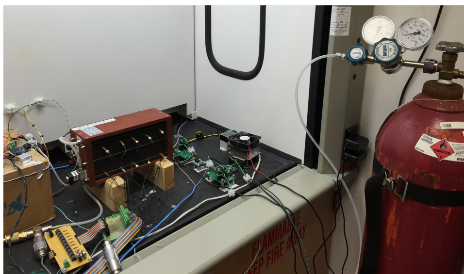
Figure 2.1. Experimental air-forced open-cathode PEMFC system.
