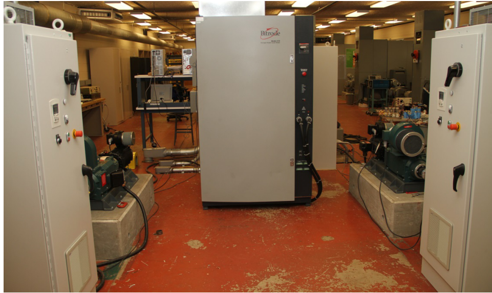
Figure 4.4. HiL test bench for emulating HEVs.
