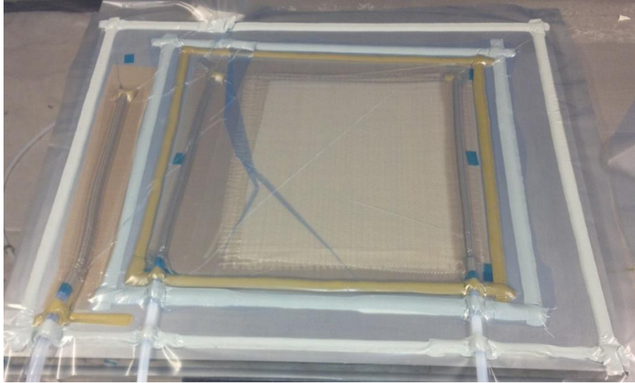
Figure 1. VARTM double bag setup with full vacuum applied before resin infiltration
