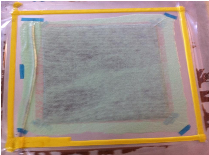
Figure 2. Image of flat panel out-of-autoclave bag setup
