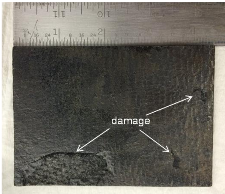
Figure 9. Optical image of \text{ZrB}_2\text{-SiC/SiC}_f sample after third PIP cycle
