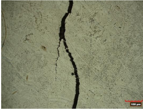
Figure 11. Optical image of a transverse cross-sectioned laser deposit showing a crack
