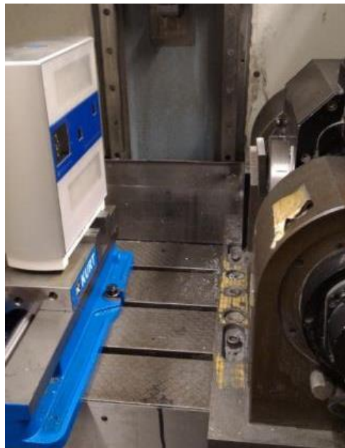
Figure 14. Scanning the part before machining
