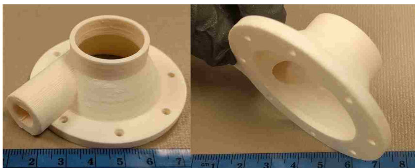
Figure 6. Final turbine-blower housing part after sintering.
