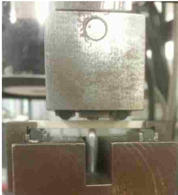
Figure 3. Fully articulating test fixture and deflectometer.
