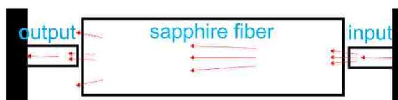
Figure 12. A schematic of losses in transmitted power as a result of input numerical aperture and diameter mismatch.
