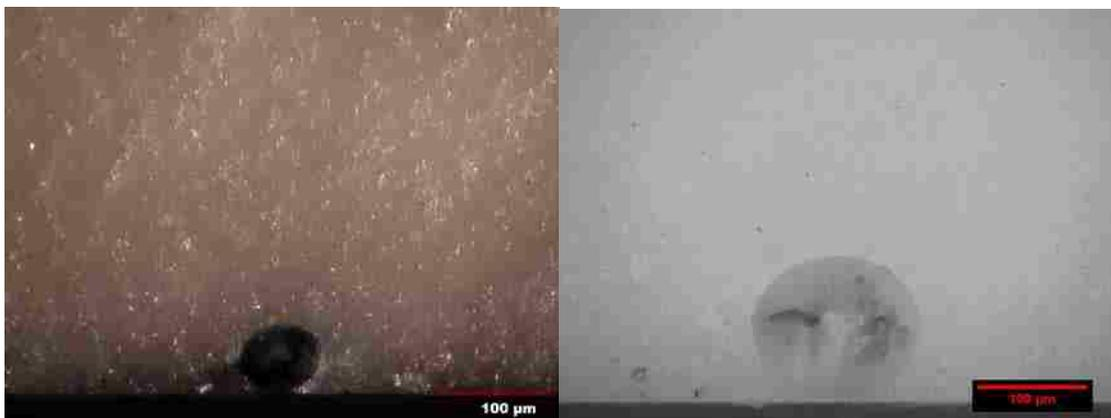
Figure 8. Two typical fracture origins near the tensile surface of the Al<sub>2</sub>O<sub>3</sub> flexure test specimens.
