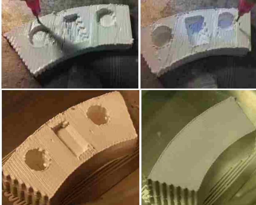
Figure 12. Liner blocks fabricated at different rastering angles.
