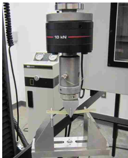
Figure 2.3. Experiment setup for three-point bending test
