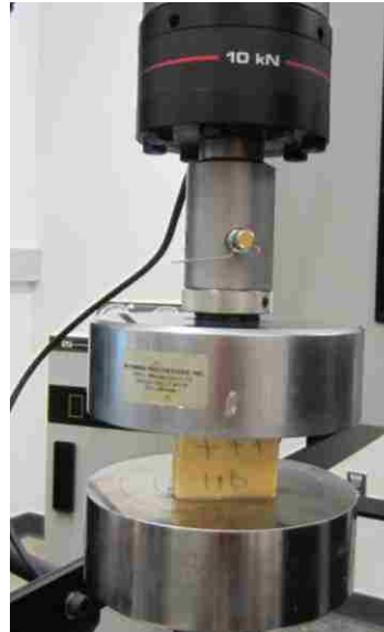
Figure 2.2. Experiment setup for compression test
