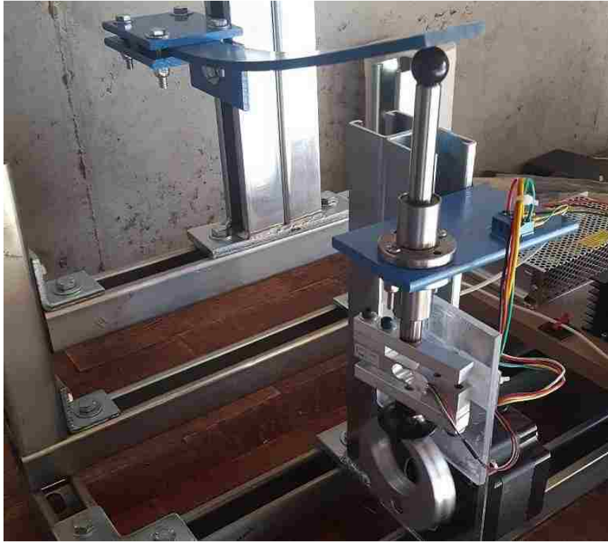
Figure 9: Homogeneous Test Specimen Shown at Maximum Displacement
