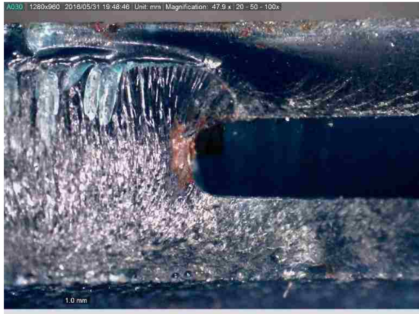
Figure 17: Fracture Surface Surrounding the Metallic Reinforcement Slot
