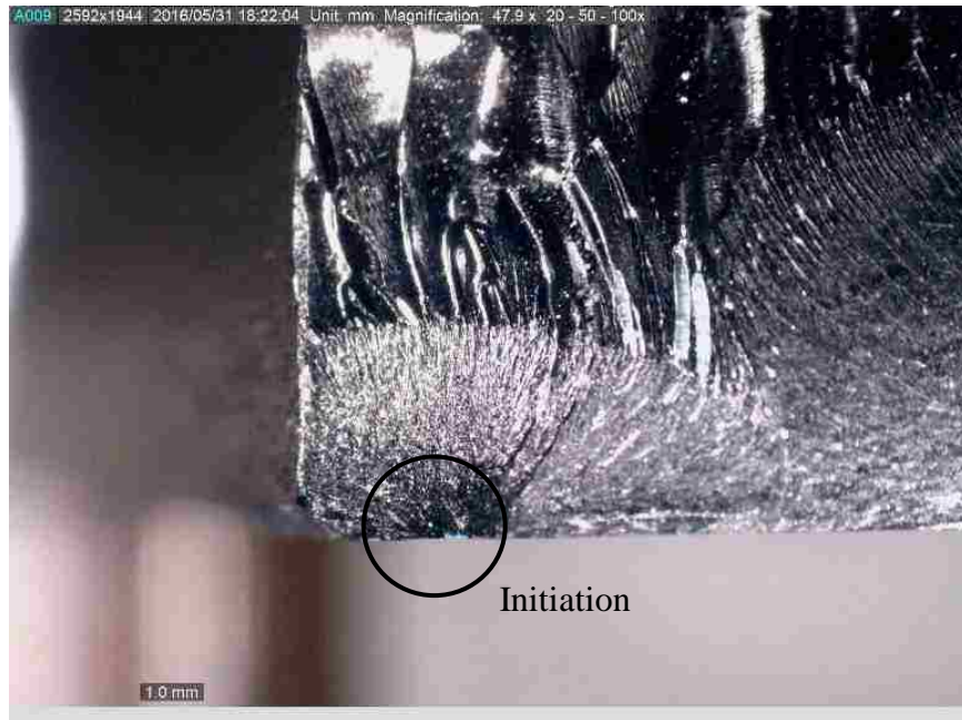
Figure 15: Close-up View of Fracture Initiation of a Homogeneous Specimen
