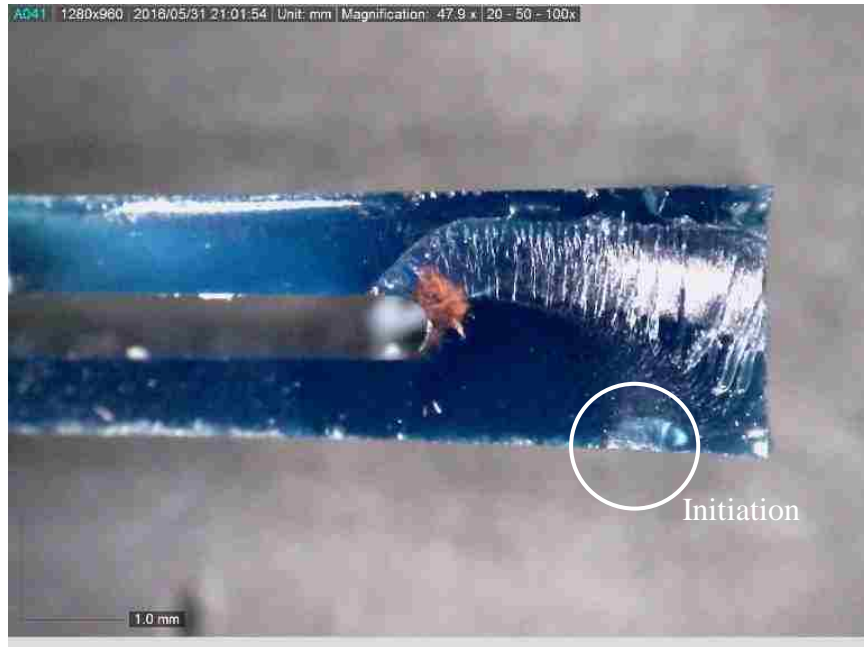
Figure 16: Fracture Initiation of a Metallic Reinforced Specimen
