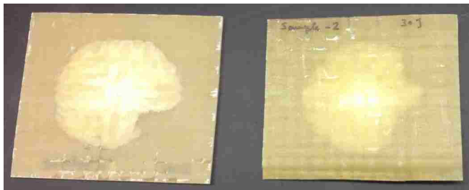
Figure 12 Shows the damaged area of glass fiber/PU90IK01
