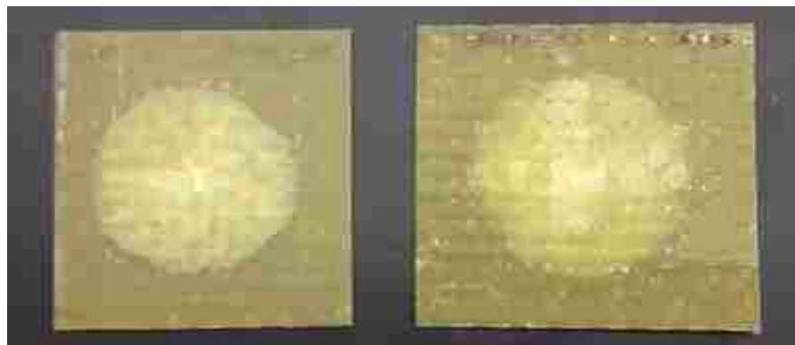
Figure 13 Shows the damaged area of glass fiber/PU 840871
