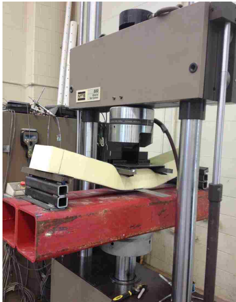
Figure 7 Shows applying bending load up to failure occurred
