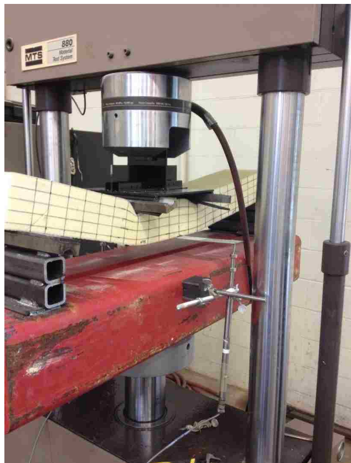
Figure 5 Shows panel deflection during the test
