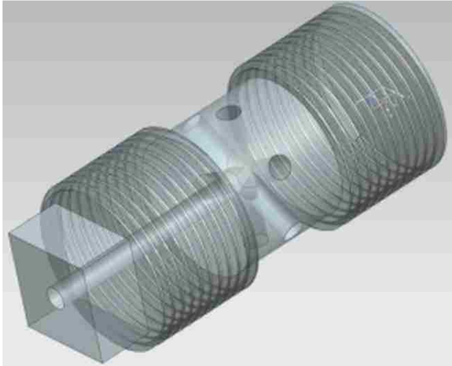
Figure 6: Internal view of manifold design in ASA (Multi point entry and exit of fuel with limited manufacturing complexity)
