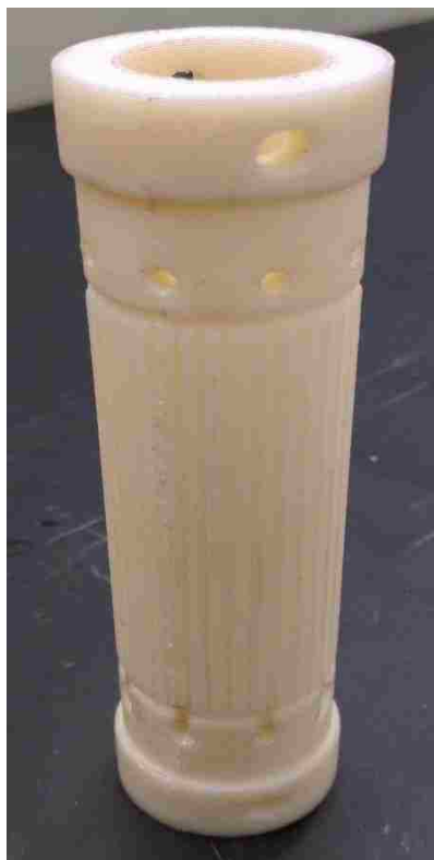
Figure 17: Chimney shaped mandrel manufactured using FDM
