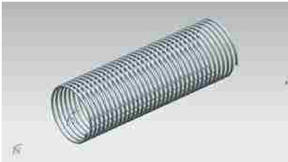
Figure 3: Helical flow sections with multiple 90° elbow bends
