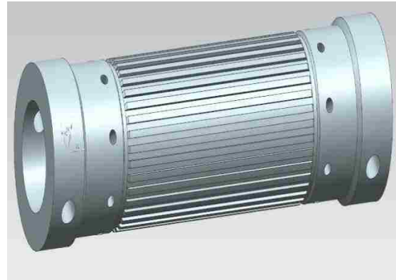
Figure 13: Mandrel sections housing fuel flow channels
