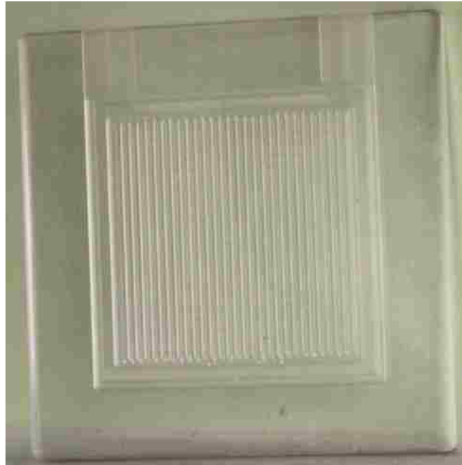
Figure 5: Hydrogen side flow plate manufactured in polycarbonate
