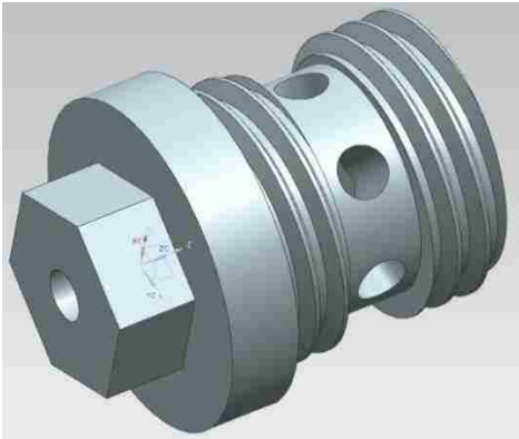
Figure 12: Inlet and exit caps designs with threads to help sealing
