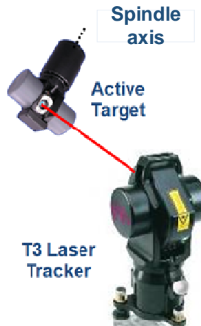
Figure 8: Illustration of laser tracker and active target.
