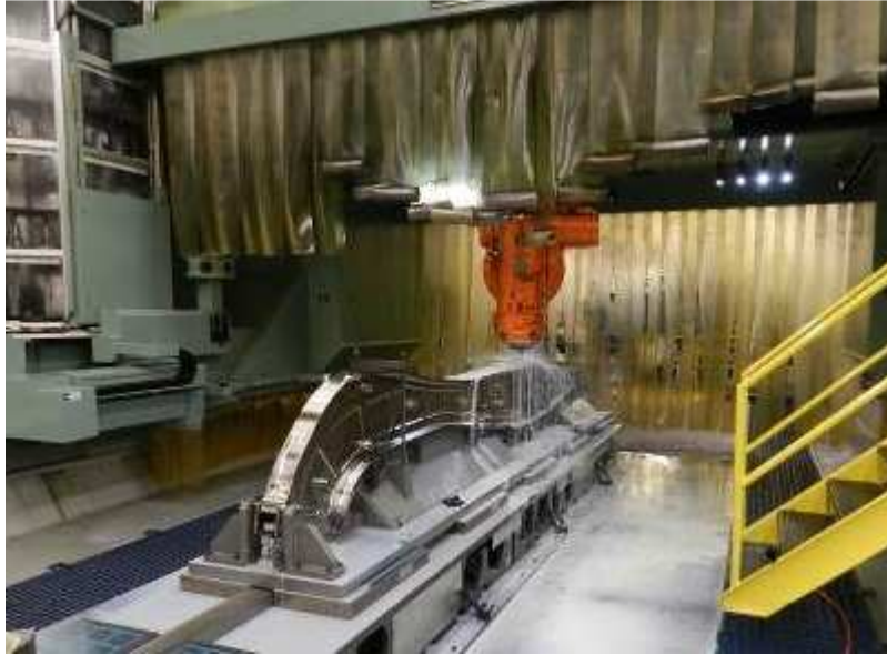
Figure 2.8: Master Mill machining a complex part.
