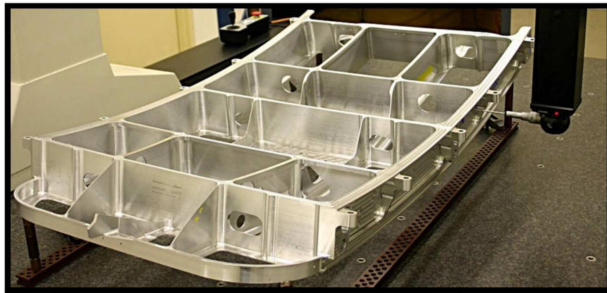
Figure 1.1: An example of a monolithic part that combines smaller components with features requiring tight tolerances.
