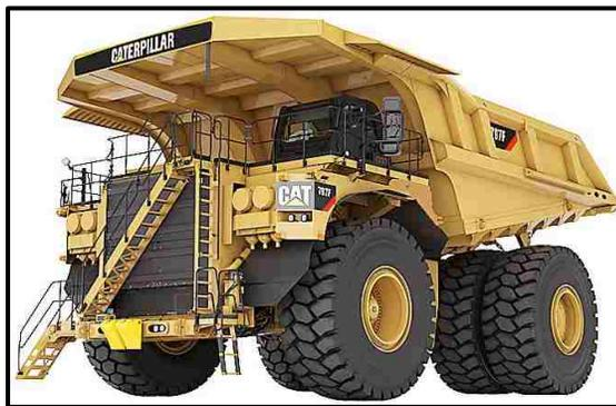
Figure 3.1 CAT 797F conventional rear dump truck [166]
