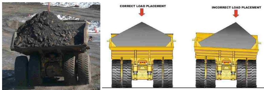
Figure 4.20 Left and right truck over-loading [178], [30]
