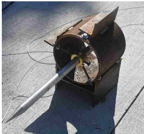
Figure 3.3. Pencil probe holder for shock tube testing
