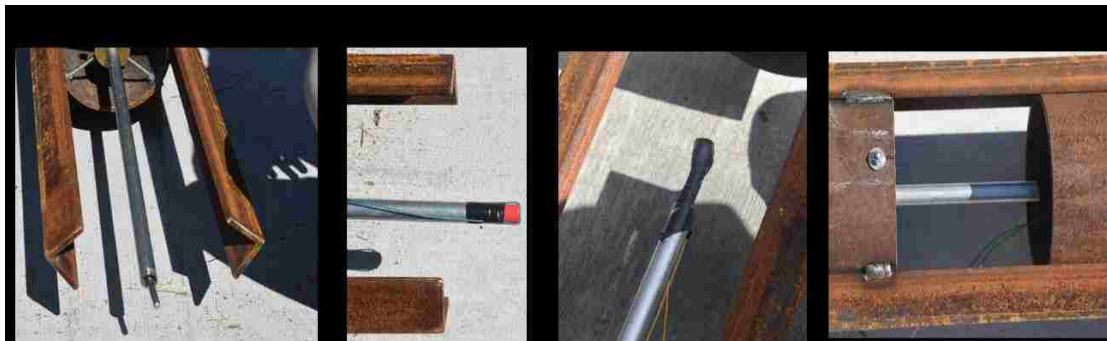
Figure 3.4. Setup of explosive charges a. Detonator b. Stinger c. C4. d. Charge inserted into shock tube
