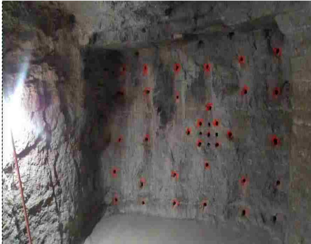
Figure 5.1. Representation of the 34 holes schematic drill pattern
