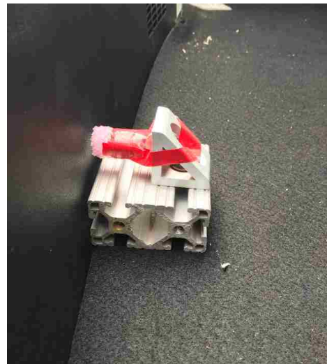
(4.10.b) Shorter source holder used for source-in-vehicle in-motion validation measurements.
