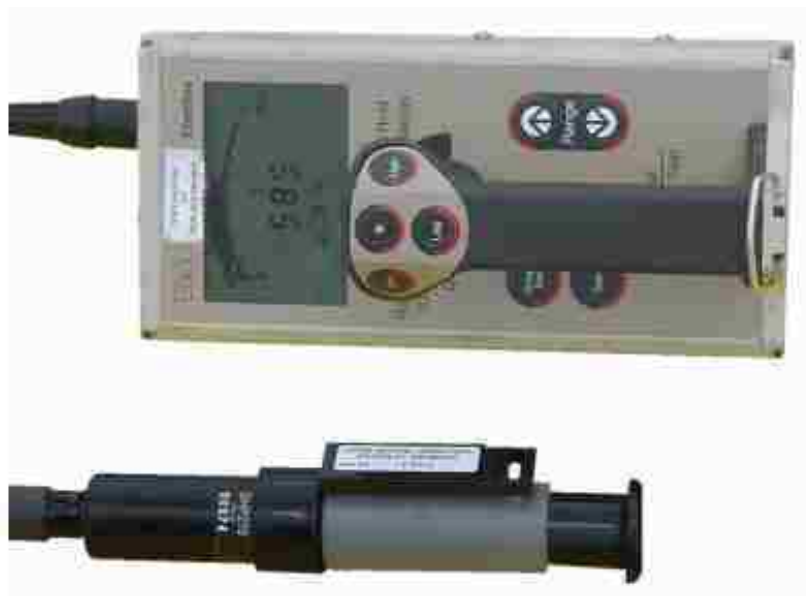
Figure 2.3: Eberline E-600 Rate meter with SHP-270 probe [23].
