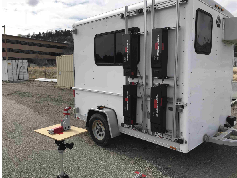
Figure 2.4: ^{147}\text{Cs} button source placed in foam source holder on top of tripod and aligned to reference detector module center.
