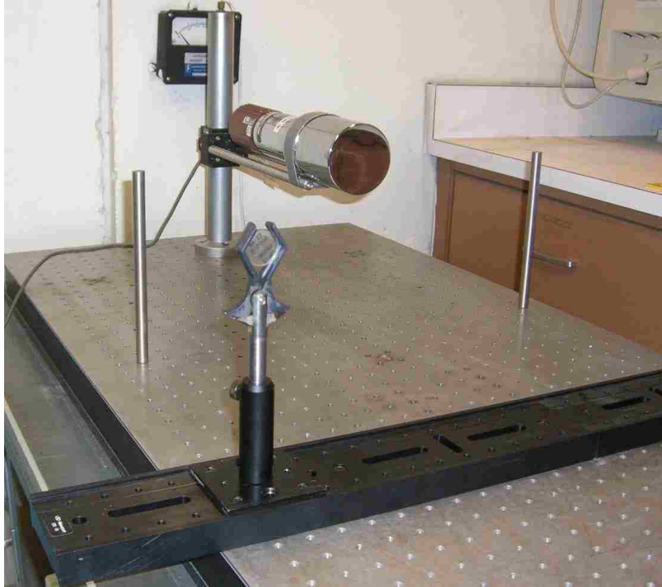
Figure 6.24 - Experimental setup for 3x3 NaI detector and source
