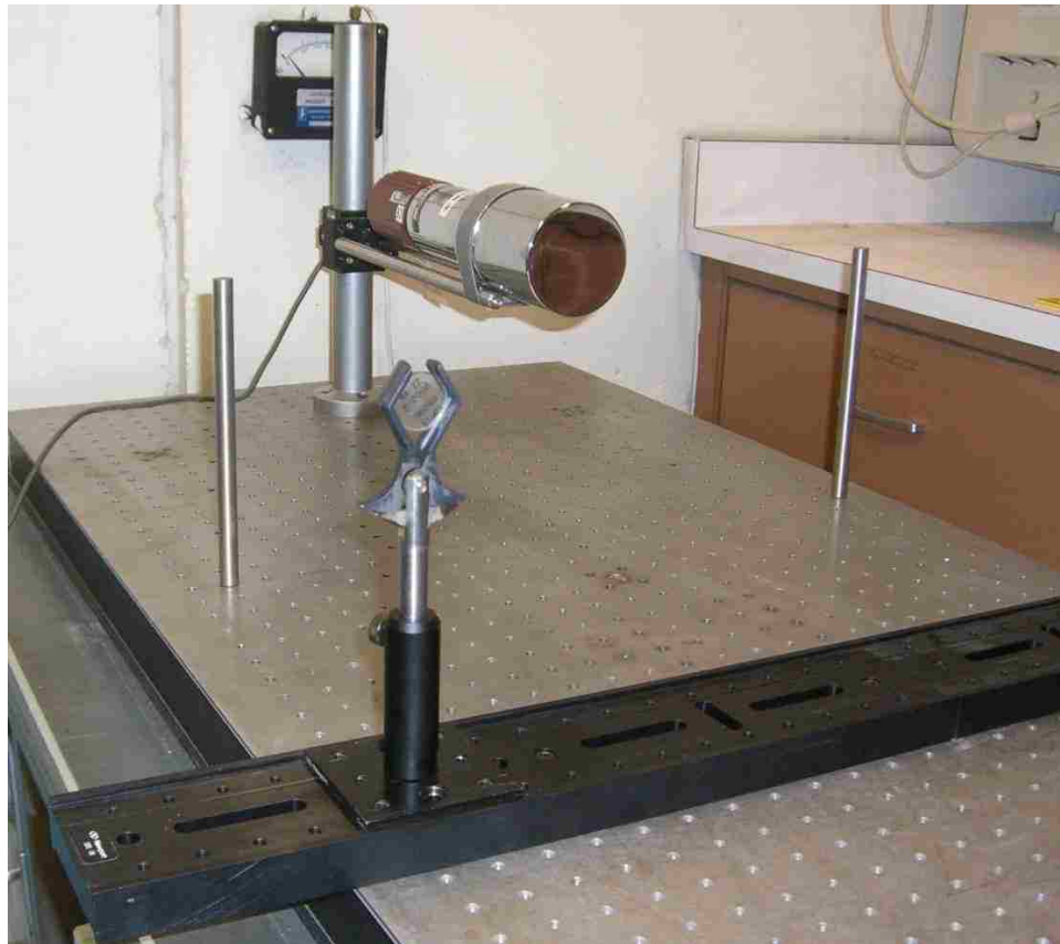
Figure 4.2 - Experimental detector with steel table and concrete wall
