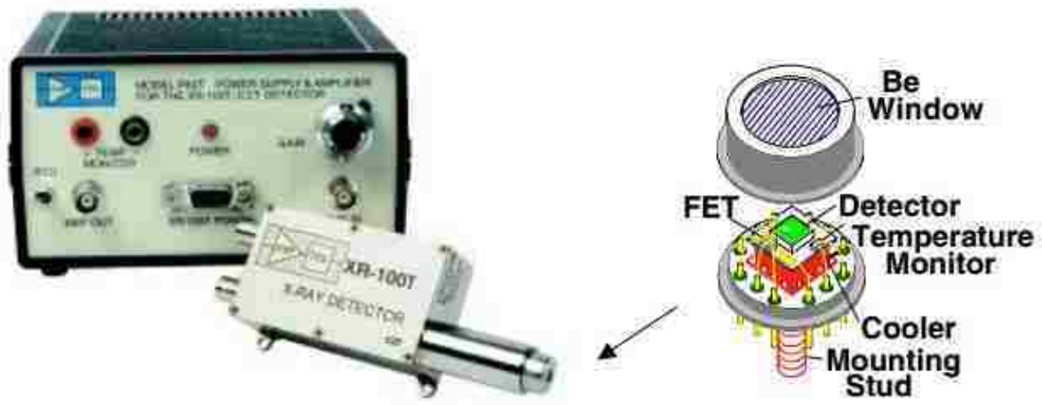
Figure 29: Amptek detector unit with power supply (right) and internal design of detector and cooler (left). [42]
