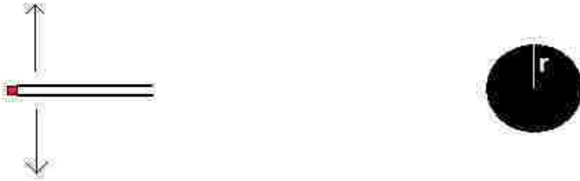
Figure 25: Basic schematic of detector (left) and source (right) in simulation. The source is shown in red with the collimator represented to the right of it. Arrows suggest directions of motion.
