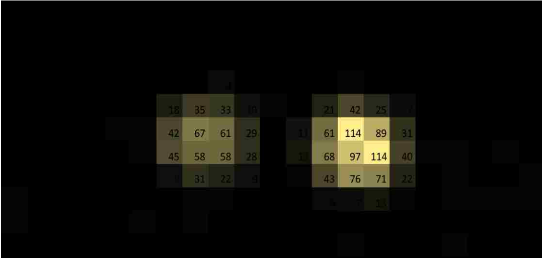
Figure 45: Two separated Eu-152 sources (3 cm apart) imaged at 30 cm from detector, at 5 minutes per pixel.
