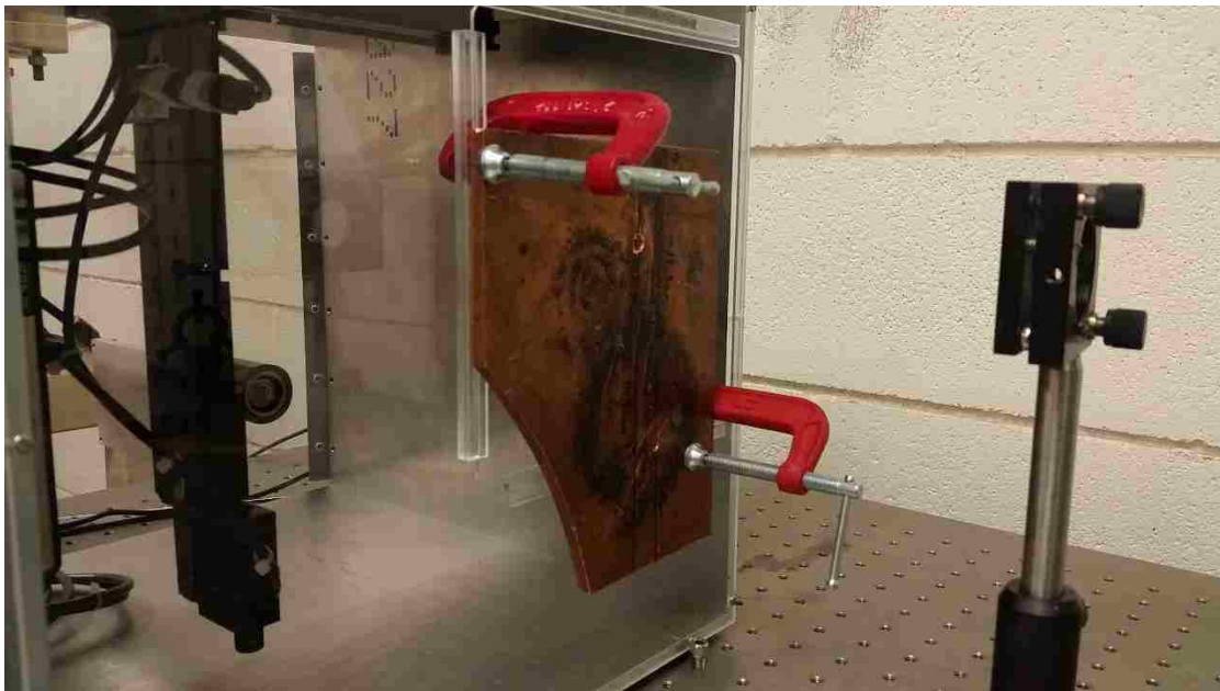
Figure 55: Experimental setup to simulate D-Matrix detector.
