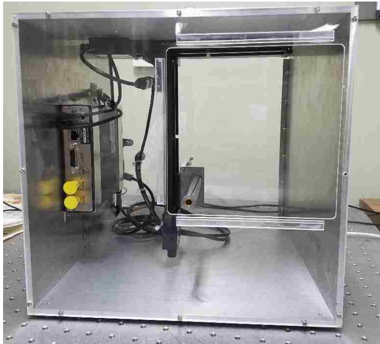
Figure 22: Nozzle collimated imaging system.
