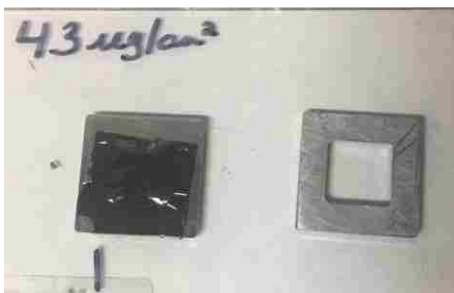
Figure 49: 43\text{ }\mu\text{g}/\text{cm}^2 carbon foil floated on frame (left) and bare aluminum frame (right).
