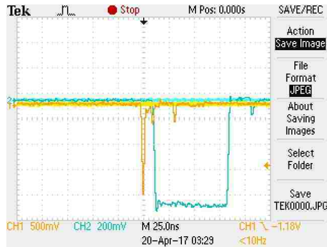
Figure 17: Oscilloscope trace of MCP signal before (orange) and after going through the discriminator (blue).
