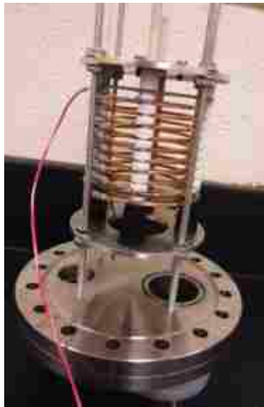
Figure 44: Axial IC installed onto ConFlat flange
