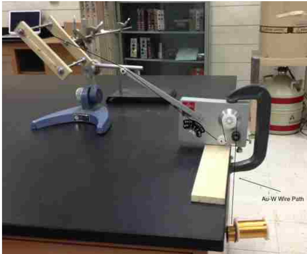
Figure 27: Au-W wire grid construction device
