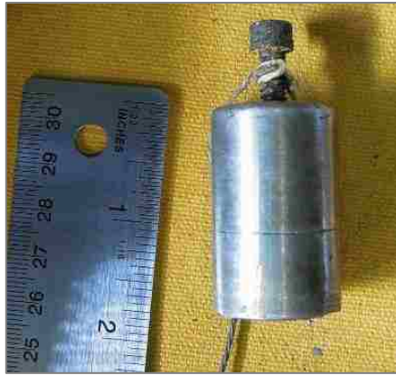
Figure 3. MRC-AmBe-44 Source Photograph and Schematic
