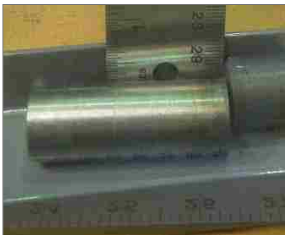
Figure 2. NB570 and NB540 ^{241}\text{AmBe} Sources Photograph and Schematic
