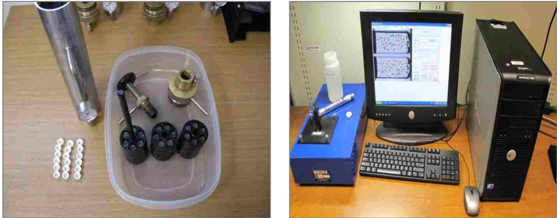
Figure 22. BDS Recompression Shielding and Reader/Bubble Counting Software
