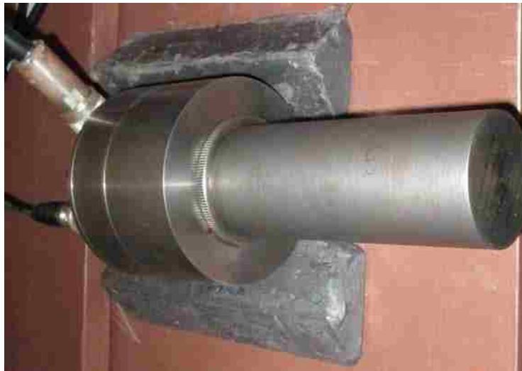
Figure 5 Re-purposed Beryllium Rod Detector Housing
