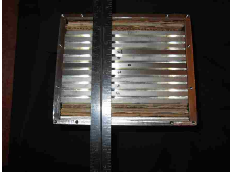
Figure 27 Active Region of Detector #2, BLC geometry Shown with .635 mm Be and 0.318 mm Scintillator
