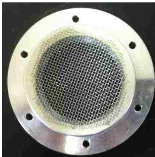
Figure 35: Original wire mesh window backing for the TOF-IC window.
