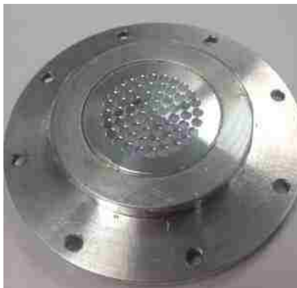
Figure 36: "Saltshaker" window backing with the surrounding window frame for the TOF-IC window. The mylar is stretched across, and epoxyed to, the window frame.
