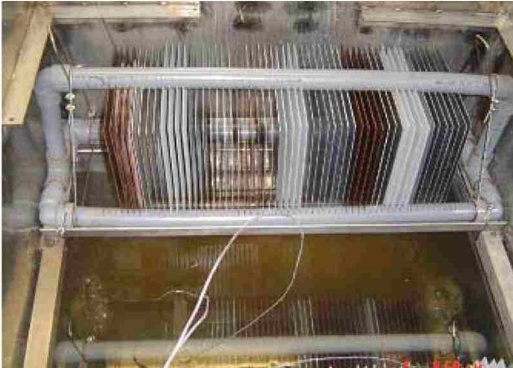
Figure 8. Metal coupon rack for the ICET experiments [16]
