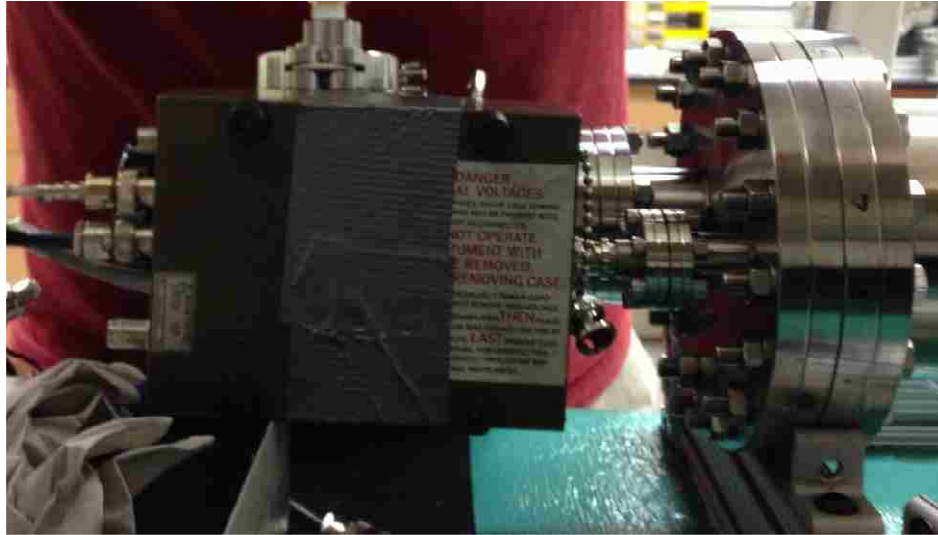
Figure 21: The preamplifier directly hooked-up to the beampipe which houses the IC
