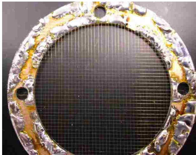
Figure 16: The mesh Frisch grid built for the various experiments
