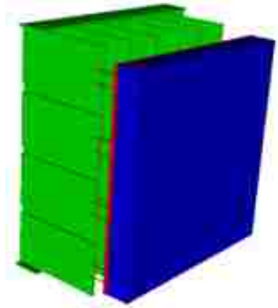
Figure 2.4: CsI array and attached preamplifiers used in the PCI (housing is omitted).
