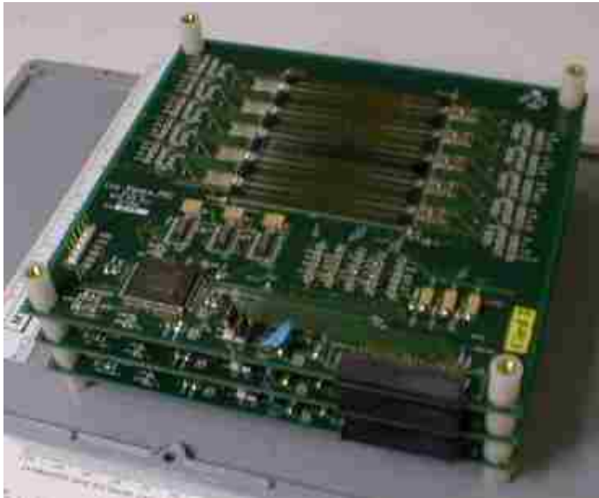
Figure 2.2: The three silicon scattering detectors stacked together with attached electronics.
