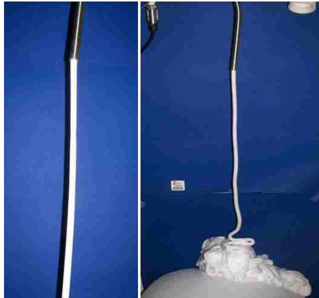
Fig. 4.33. Sequence of homogeneous foam flow within low-quality regime at 0.5 inch pipe outlet at foam quality below 99%.
