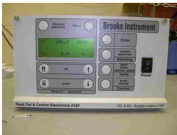
Fig. 3.6. Brooks microprocessor flow control unit
