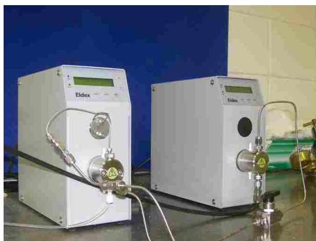
Fig. 3.7. Positive displacement Optos pumps
