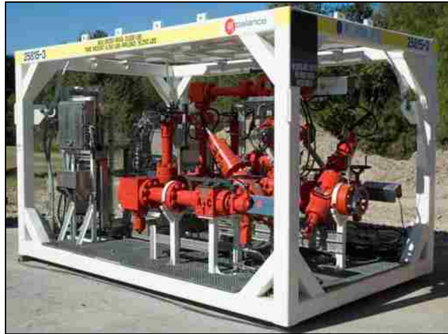
Fig. 2.3: A typical automated DCM (With the permission of AT BALANCE™)
