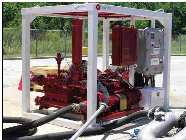
Fig. 2.7: Back pressure pump (With the permission of AT BALANCE™)
