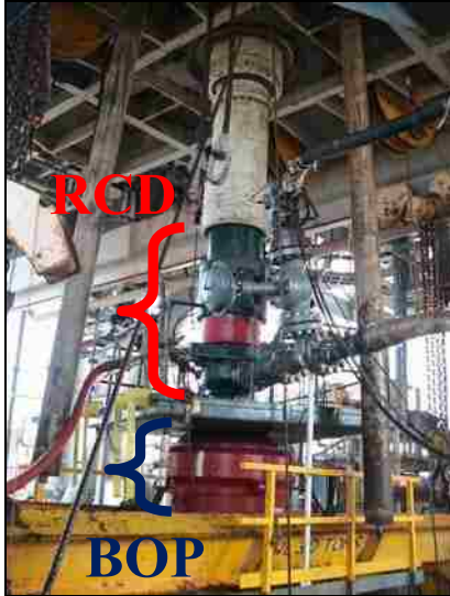
Fig. 2.2: RCD above the BOP (With the permission of AT BALANCE™)
