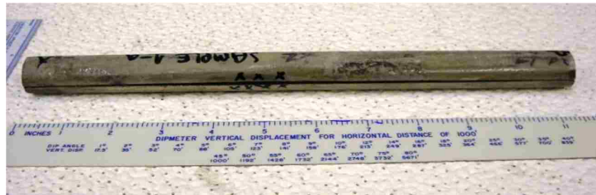
Figure 3.3: Cement Core (1 in by 12 in)
