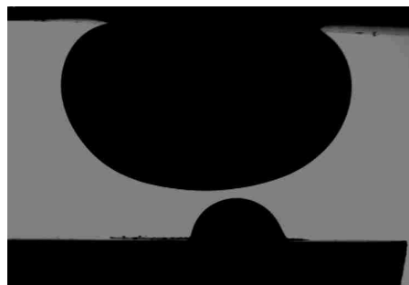
Figure 4.18: Fraction of sessile oil drop left on the lower mineral surface in the DDDC test
