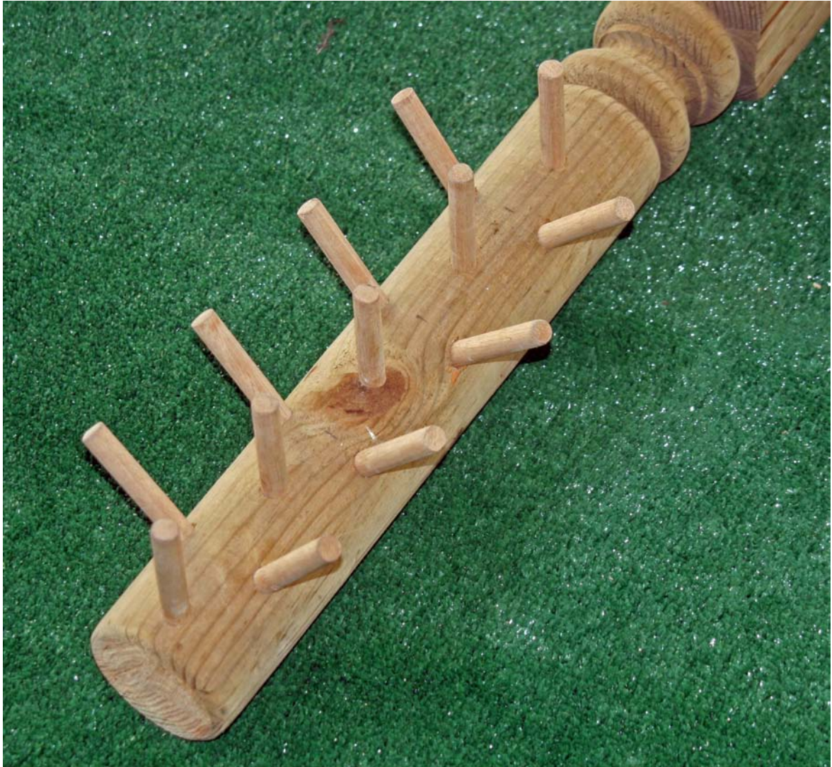
Figure 2.1. Main dowel used during gap bridging trials. The pegged surface was 40.0 cm long and 7.6 cm in diameter. Dowels of 7.5 cm in length and 1.3 cm in diameter were placed on 8.0 cm centers along the main dowel orientated at vertical and approximately 45°.
