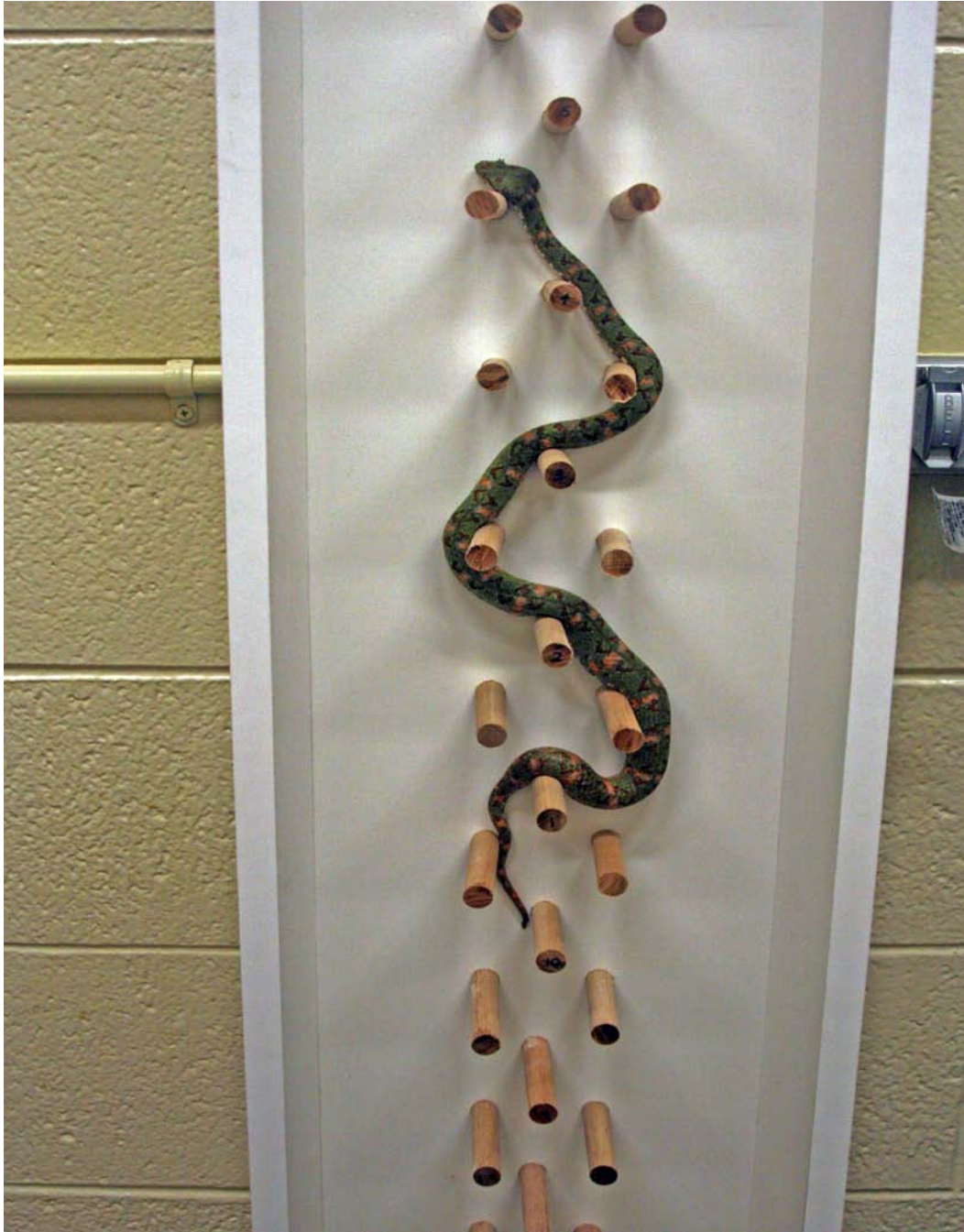
Figure 3.1. Vertical peg array. The peg array stood 2.30 m high. The pegs were 1.59 cm diameter wooden dowels that extended outward 7.50 cm. The vertical distance between single dowel rows was 10.16 cm, and the center to center horizontal distance between dowels in the same row was 6.35 cm.
